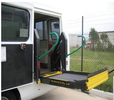
Side Loading Hoist
